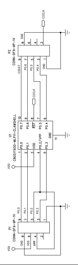
Figure 10. C8051T600 QFN Socket Daughter Board Schematic
